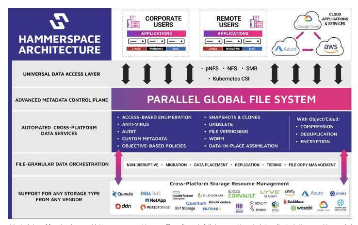
A logical view of functional areas with Hammerspace architecture. The software is fully integrated in a single installer, including everything needed to get up and running on commodity hardware, VMs or in the cloud.
